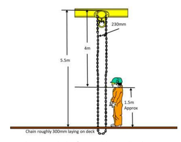
During the pre-use checks of a geared beam trolley the movement chain disengaged from the trolley guide wheel and fell 5.5 meters to the deck. The dropped chain contacted an individual by a glancing blow to the shoulder.
